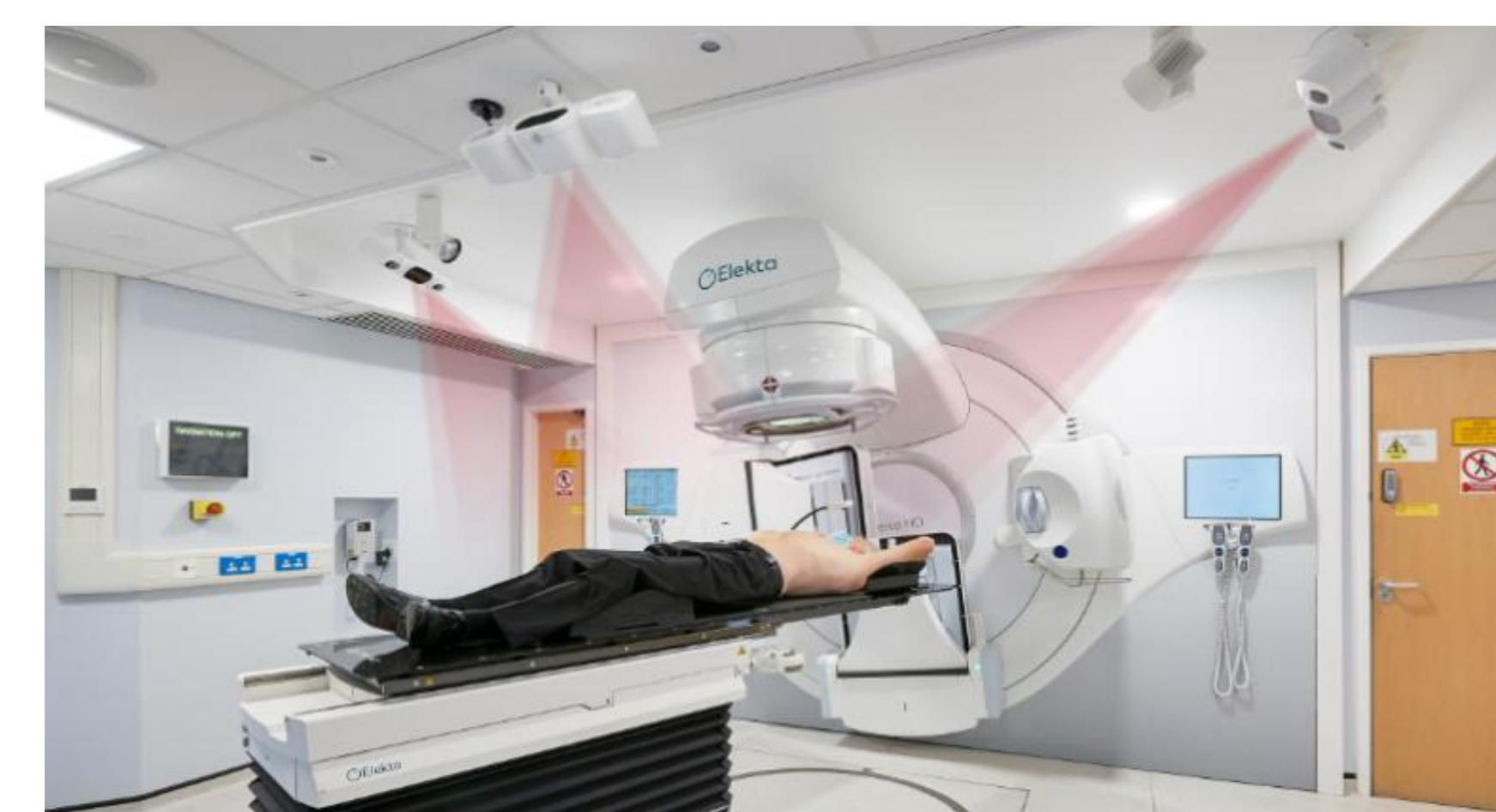
AlignRT system cameras tracking their position for precise radiation therapy delivery (Vision RT, 2026).
