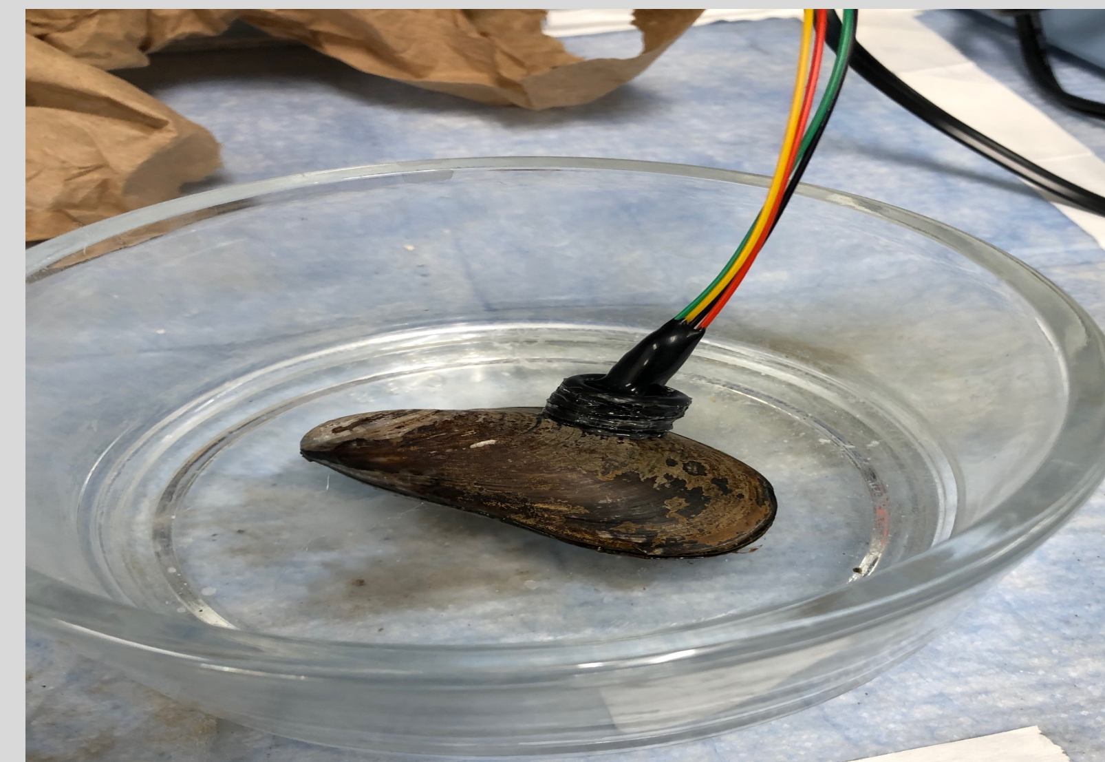
Figure 5: Heart rate sensor connected to the mussel and secured by O-rings
