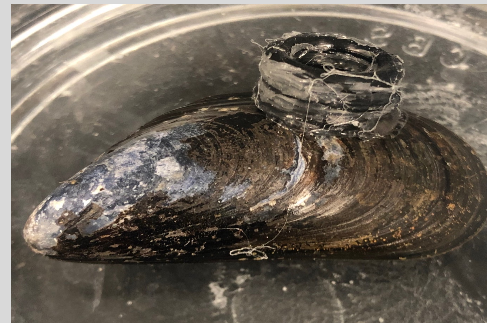
Figure 4: O-rings hot glued to heartrate location on posterior side of mussel
