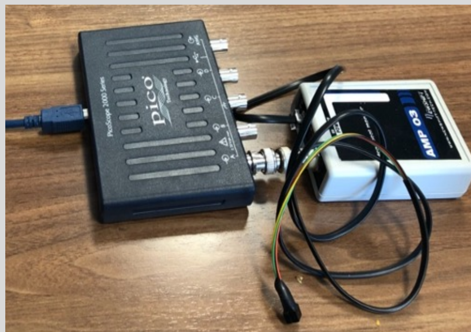
Figure 2: PicoScope2405 oscilloscope connected to heartbeat monitor
